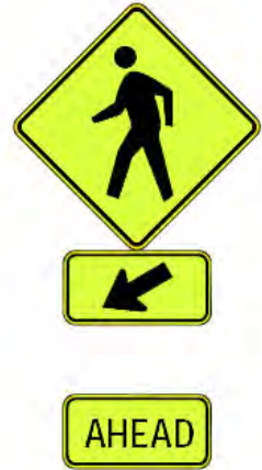
W11-2 shown with W16-7P (downward diagonal arrow) and W16-9P (AHEAD)
