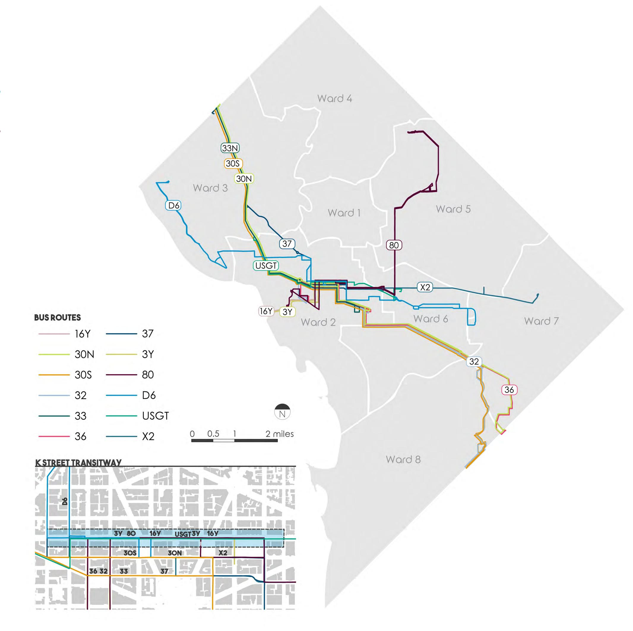
The transitway is designed to have 12 bus routes with 55 buses/hour per direction in peak period.
