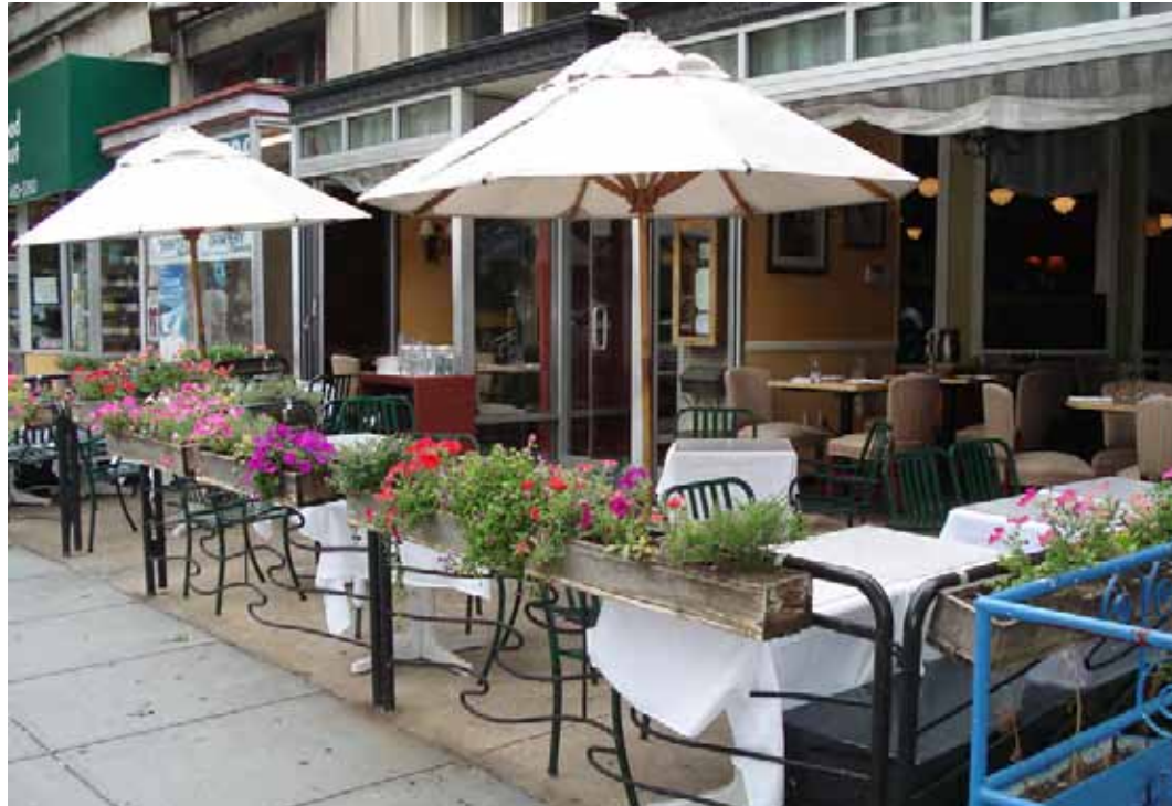
Fencing and railings around a sidewalk café shall not be higher than 36 inches.
