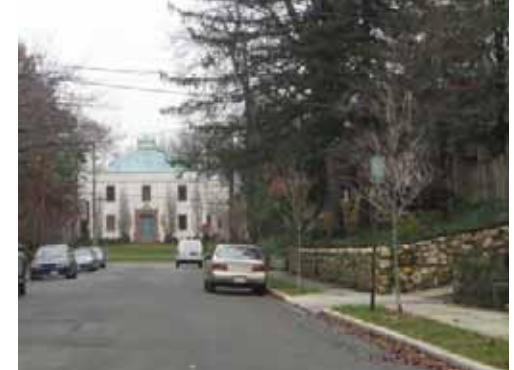
The minimum roadway width for a two-way street with parking on both sides is 32 feet.
