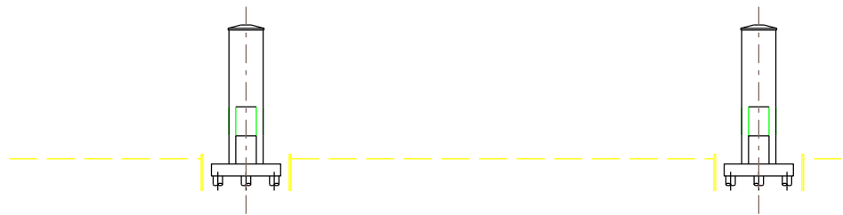
Step 1: Install cofferdam. Construct substructure, pier, and tower.
