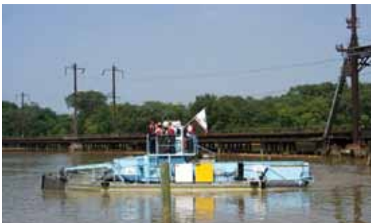
DC Water's trash skimmer boat
