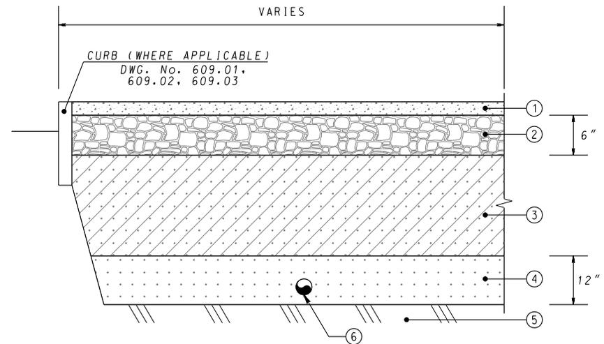
**STRUCTURAL SOIL OVER SAND WITH DRAIN OVER SCARIFIED SOIL**
