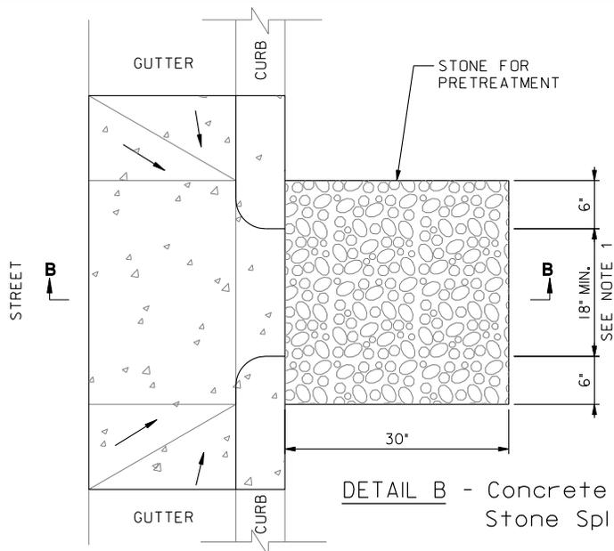
DETAIL B - Concrete Flume with Stone Splash Pad
