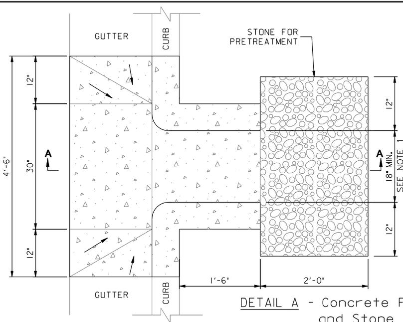
DETAIL A - Concrete Flume with Wingwalls and Stone Splash Pad
