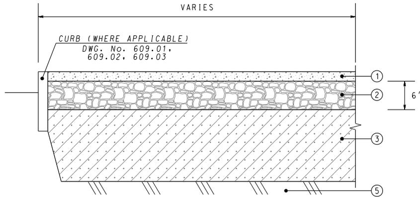
**STRUCTURAL SOIL OVER SCARIFIED SOIL**
