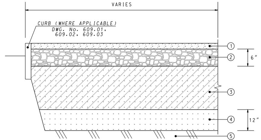
**STRUCTURAL SOIL OVER SAND OVER SCARIFIED SOIL**
