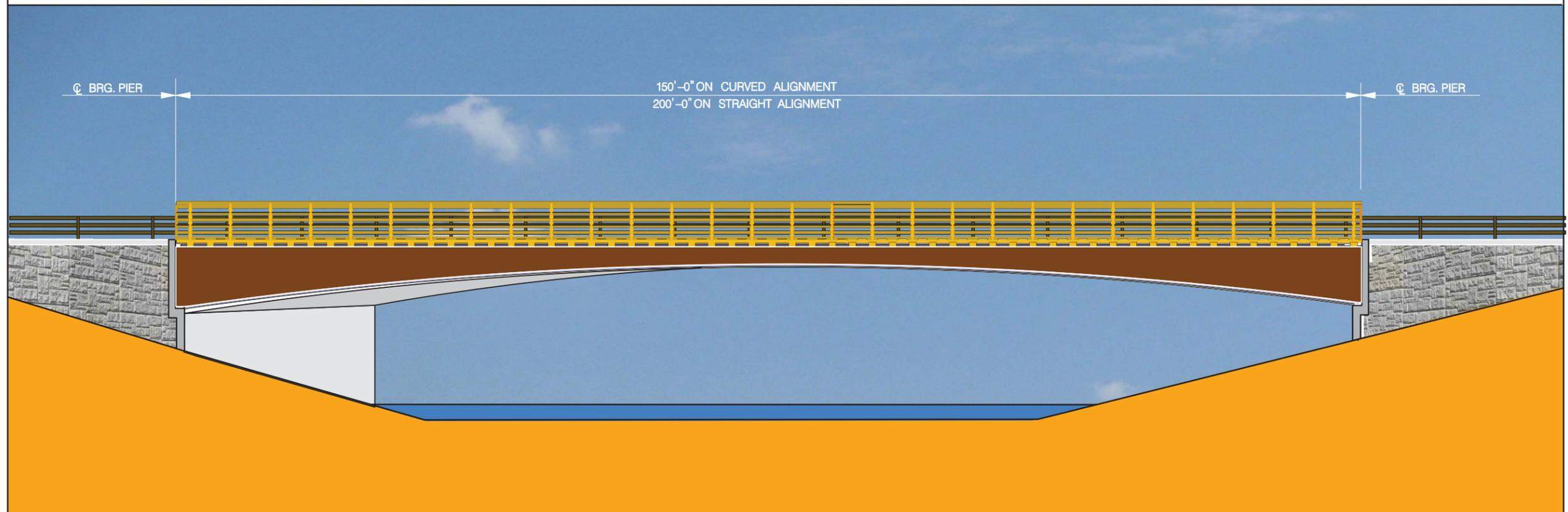
**BRIDGE OPTION 2 – STEEL BOX GIRDER WITH TIMBER FLOOR AND TIMBER RAIL**
