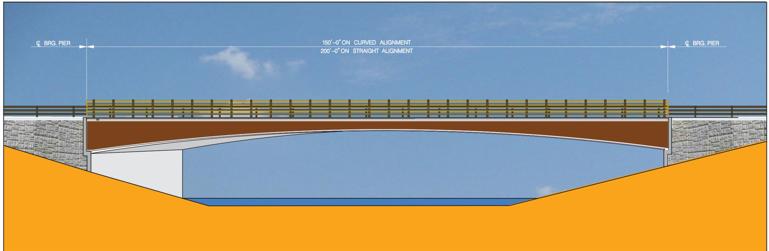
**BRIDGE OPTION 3 – STEEL BOX GIRDER WITH CONCRETE FLOOR AND STEEL RAIL**
