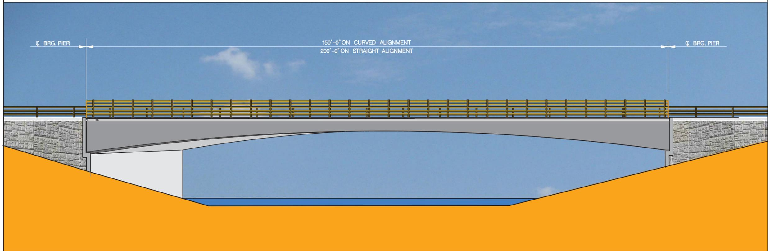
**BRIDGE OPTION 4 – CONCRETE BOX GIRDER WITH CONCRETE FLOOR AND STEEL RAIL**
