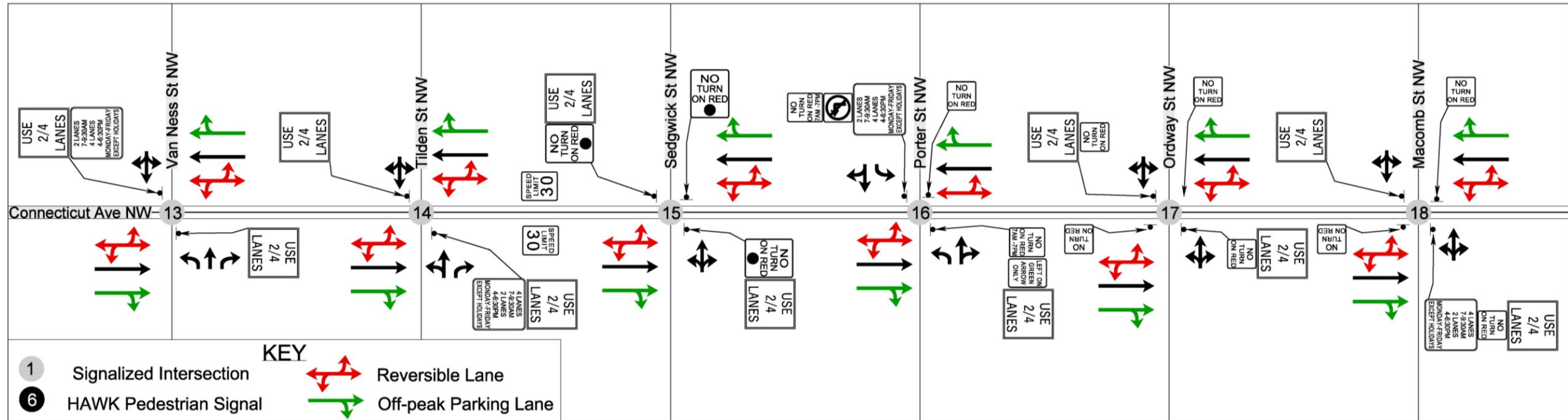
Figure 10: Traffic Control, Operational Signage, Parking, and Lane Geometry from Devonshire Place NW to Calvert Street NW
