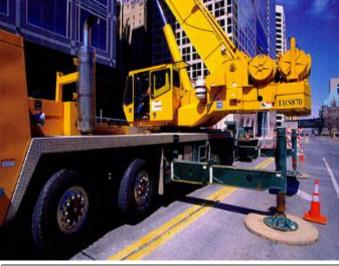
Outriggers are extended legs of mobile cranes that take load from wheels during lifting stage.
