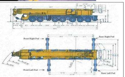
The Basic Dimensions for a 400-ton crane
