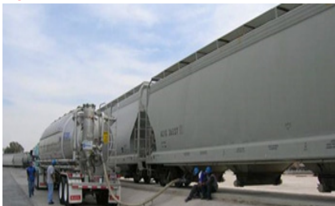
Figure 16: Bulk Transload from Railcar to Truck
