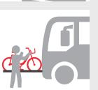
3. Lift the bicycle onto the rack, placing it into one of the slots. There is a spring-loaded support arm attached to each bike space.
