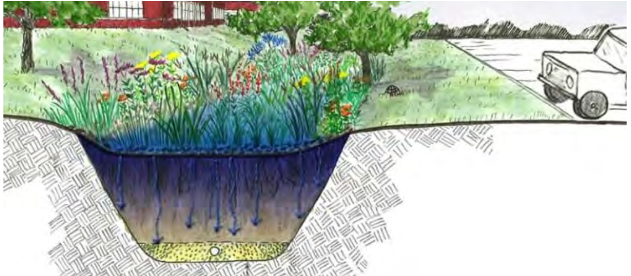
Diagram of a Bioswale / Rain Garden
