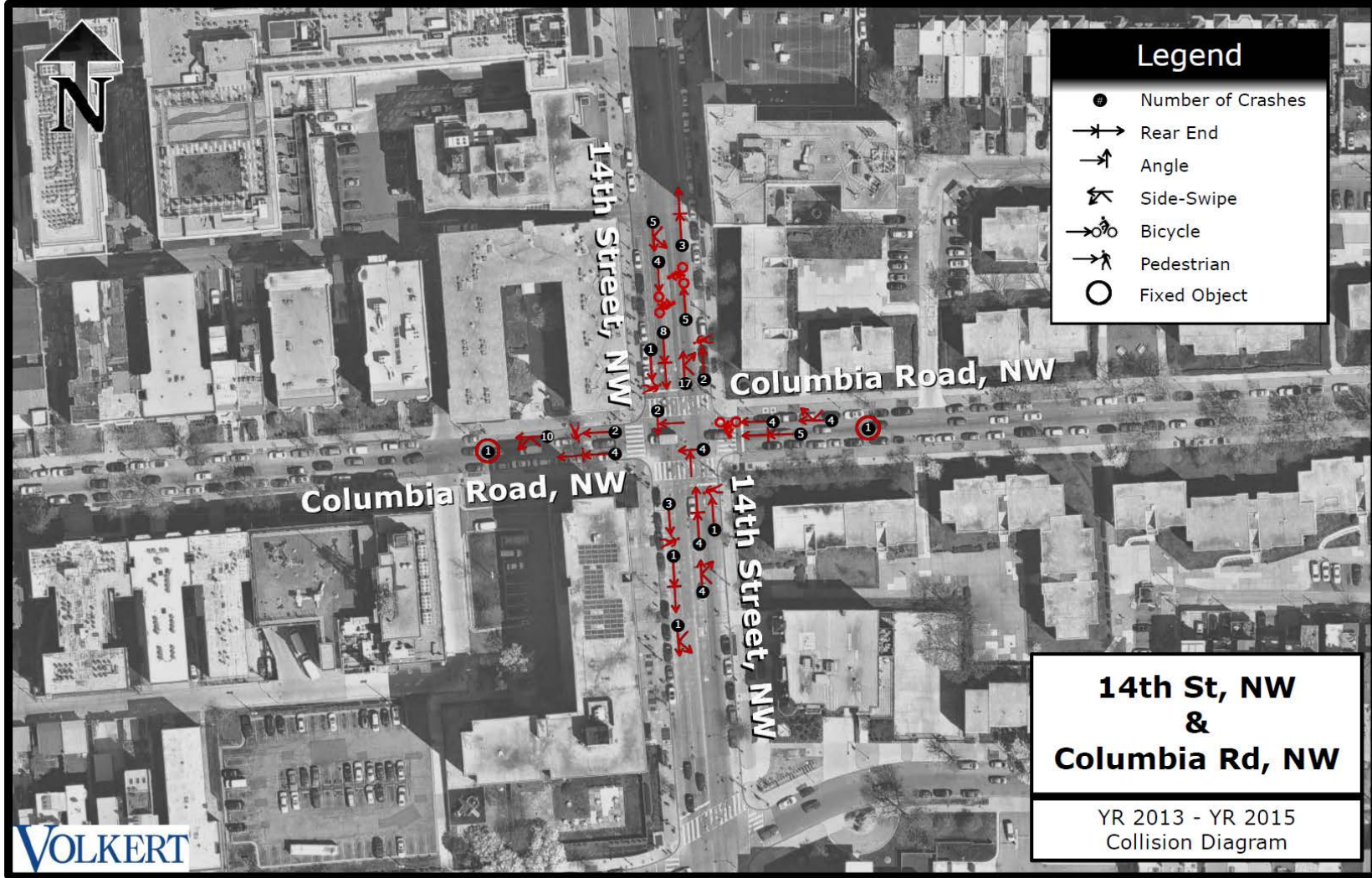
Figure 10. 14th Street and Columbia Road NW Crash Diagram
