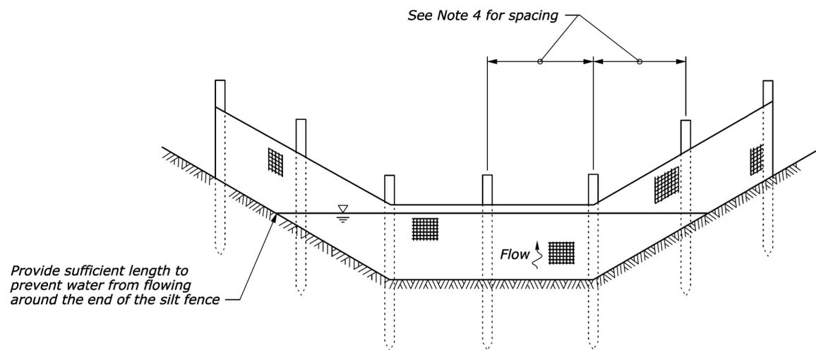
**SILT FENCE INSTALLATION IN A DRAINAGE DITCH**
