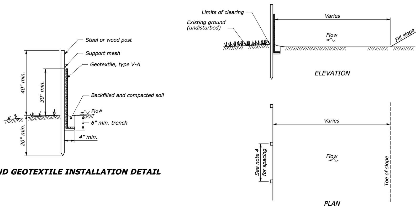
**POST AND GEOTEXTILE INSTALLATION DETAIL**
