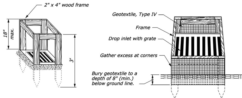
**SILT FENCE DROP INLET PROTECTION (TYPE A)**
