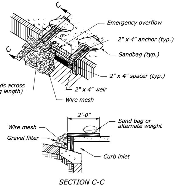
**CURB INLET PROTECTION, WOODEN WEIR (TYPE E)**
