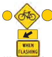
Bicycle Warning Sign W11-1 with Plaque W16-7P, W16-13P and Flashers
