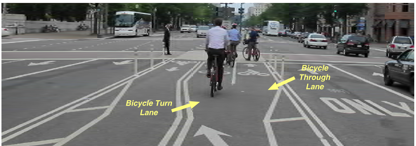
WESTBOUND 6TH STREET INTERSECTION STRIPING FIGURE 4C
