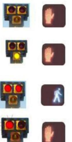
**Sequence 1:** Blank Signals upon activation with Steady Don't Walk
