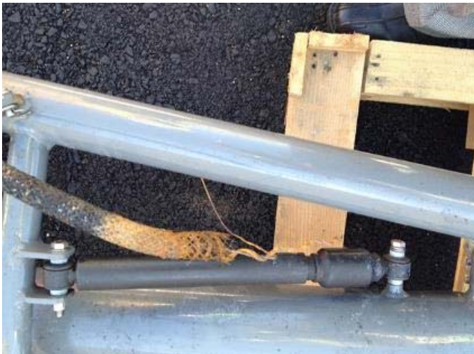
(Figure 3 - Fire damage on car 202 showing the burnt cable on the pantograph.)
