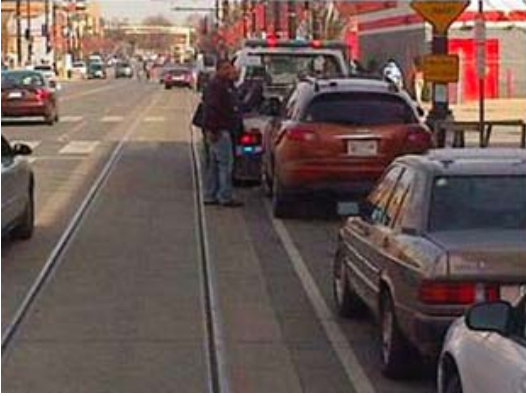
( Figure 12 – Issues of automobiles infringing on the dynamic envelope of the streetcar)
