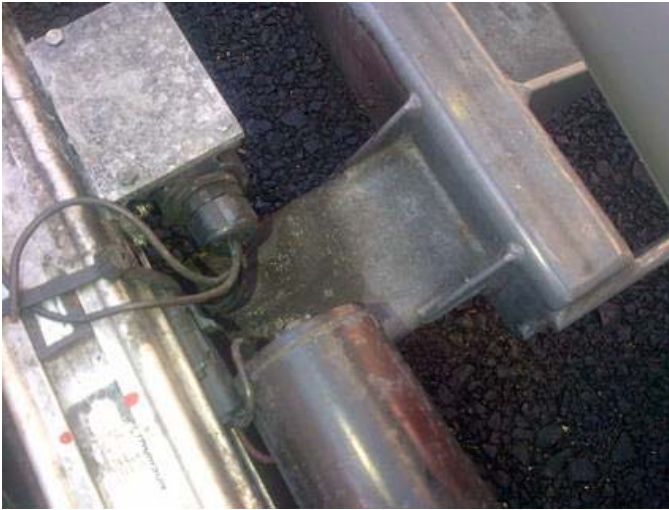
(Figure 2 - Pantograph component damaged in the fire on car #202 on February 21, 2015.)
